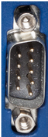
Pin assignment 9-pole Sub-D plug
